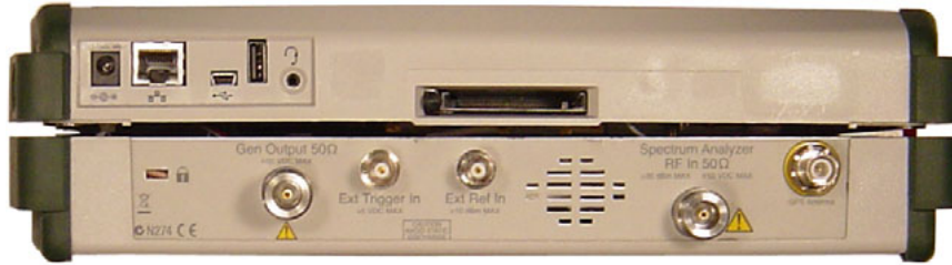
Figure 3-6. MS272xB Case Halves Partially Separated
